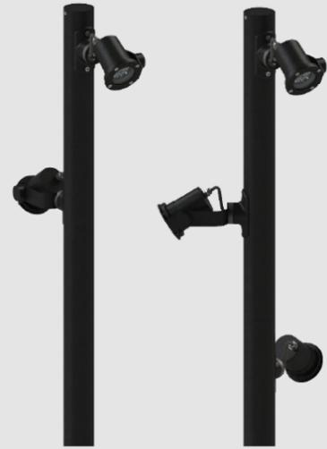
POSTE COM PROJETOR ORIENTÁVEL COM TECNOLOGIA LED . USO EXTERNO. CORPO EM ALUMÍNIO INJETADO, ARO EM AÇO INOX AISI 316 E VIDRO TEMPERADO DE 10MM. ÍNDICE DE PROTEÇÃO IP67. ÍNDICE DE RESISTÊNCIA MECÂNICA IK09. INCLUI DRIVER ALOJADO NO CORPO DA LUMINÁRIA E ANEL ANTIOFUSCANTE.
